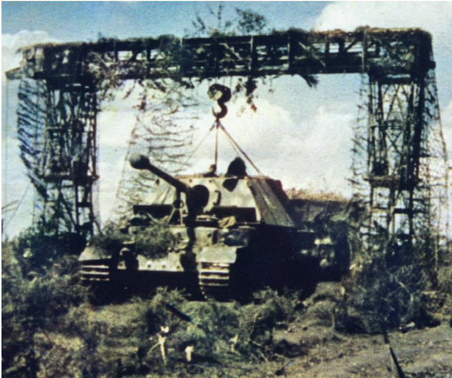
German repair crews hoist the turret of an Elephant tank destroyer using a gantry crane during operations in the Soviet Union. Damage from mines and mechanical failure made it essential to have forward-deployed repair facilities.
