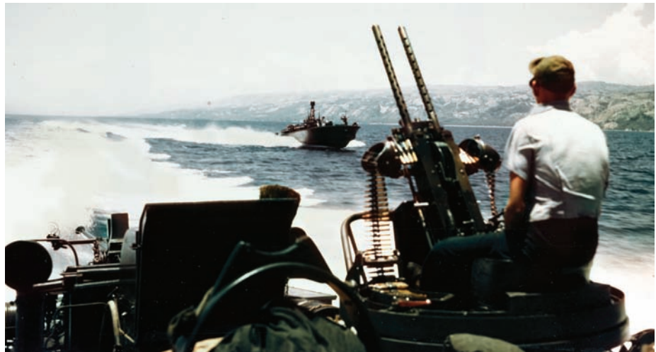
ABOVE: PT boats go into action in support of U.S. forces participating in the landings on Mindanao Island in the Philippines. PT boats, which were designed to intercept ships of larger classes, were armed with torpedoes, cannons, rocket launchers, and dual .50-caliber machine guns. BELOW: During the island hopping in the Pacific, PT boats blocked enemy vessels shelling U.S. positions and intercepted Japanese vessels transporting troops to islands.
