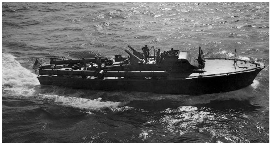
ABOVE: PT boats go into action in support of U.S. forces participating in the landings on Mindanao Island in the Philippines. PT boats, which were designed to intercept ships of larger classes, were armed with torpedoes, cannons, rocket launchers, and dual .50-caliber machine guns. BELOW: During the island hopping in the Pacific, PT boats blocked enemy vessels shelling U.S. positions and intercepted Japanese vessels transporting troops to islands.
