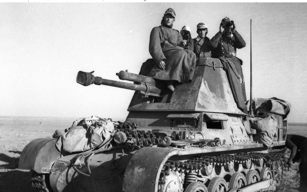
ABOVE: German soldiers man a Panzerjäger I in the Libyan desert near Bardia. Mounting a 47mm anti-tank weapon atop the chassis of the Panzer I tank, the Panzerjäger I was among several tank destroyer/assault gun vehicles developed by the Germans during World War II. OPPOSITE: Bayonet-wielding Australian troops rush through the ruined streets of Bardia in search of stray Axis soldiers.
