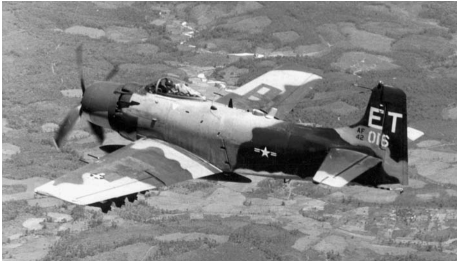
The propeller-driven Douglas A-1 Skyraider, armed with four 20mm cannons and capable of carrying 8,000 pounds of external ordnance, could remain on station over a target much longer than a jet.
