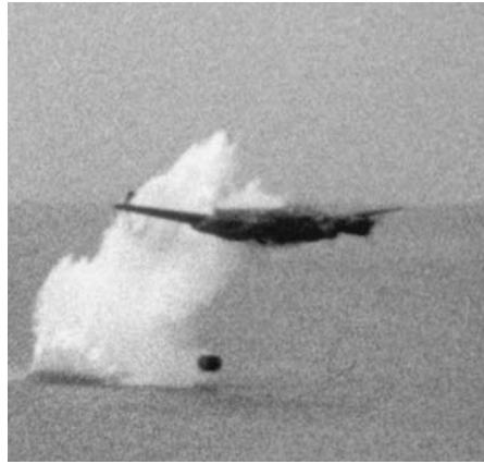
LEFT: An 8,850-pound Upkeep bomb is shown tethered to the belly of a Lancaster in preparation for the raid. MIDDLE: When a Lancaster released a dummy Upkeep bomb during a practice run at Reculver bombing range, the water plume damaged the aircraft. RIGHT: Inventor Barnes Wallis and RAF personnel watch as the dummy bomb skips toward the shoreline.
