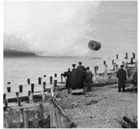
LEFT: An 8,850-pound Upkeep bomb is shown tethered to the belly of a Lancaster in preparation for the raid. MIDDLE: When a Lancaster released a dummy Upkeep bomb during a practice run at Reculver bombing range, the water plume damaged the aircraft. RIGHT: Inventor Barnes Wallis and RAF personnel watch as the dummy bomb skips toward the shoreline.
