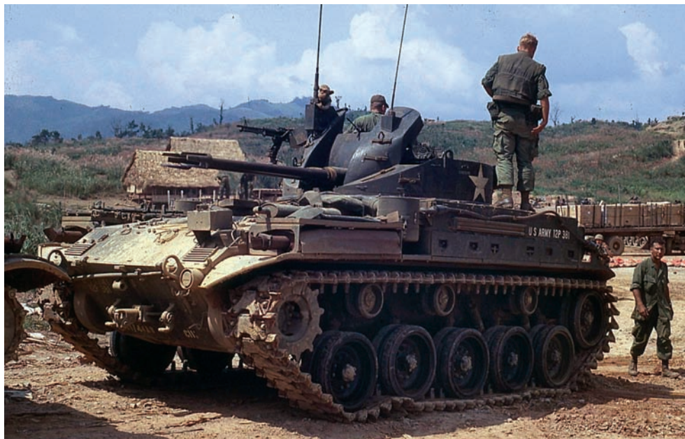
ABOVE: Marine commanders relied on the M42A1's firepower for harassment-and-interdiction missions. This M42A1 defends a section of the vital Route 9 corridor from Dong Ha to Khe Sanh in 1968. OPPOSITE: A soldier takes aim through an M42A1 Duster gun sight at Fort Bliss, Texas in 1982. After more than three decades in service, the U.S. Army retired the venerable self-propelled anti-aircraft gun in 1988.
