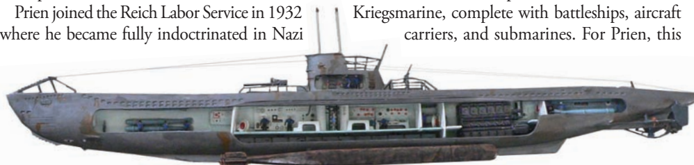
ABOVE: The Type VII B U-boat, which carried 14 torpedoes, boasted powerful engines and two rudders for enhanced agility. TOP LEFT: Captain Gunther Prien. TOP RIGHT: Crewmen line the conning tower of U-47. The submarine sank three British merchant ships in the first week of September 1939.
