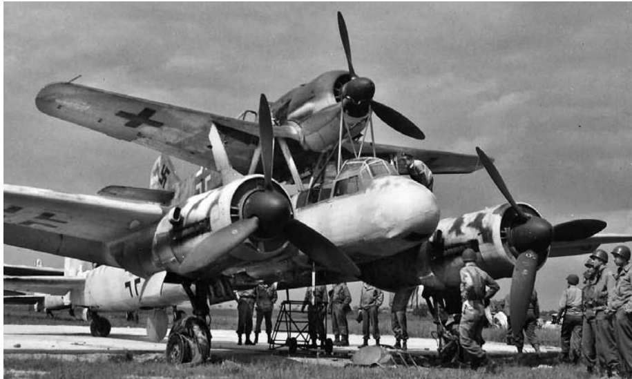
The Mistel composite aircraft consisted of an Fw-190 fighter attached to a Junkers Ju-88 bomber. U.S. soldiers inspect this captured example at an airbase in Bernberg, Germany, in the spring of 1945.
