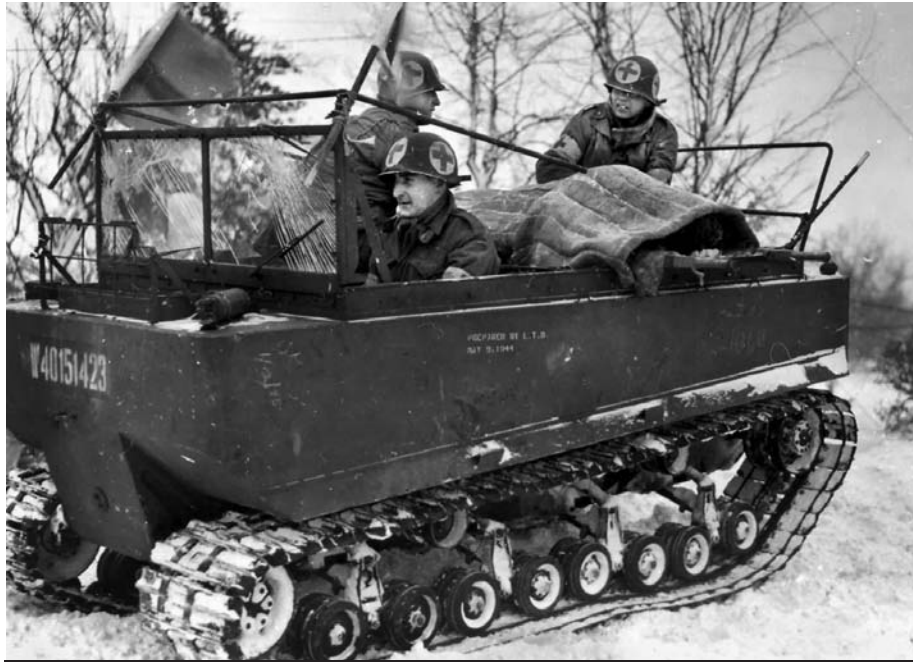
The M29 Weasel, a tracked vehicle made for operations in winter weather, was suggested by Pyke. This example belongs to the 79th Infantry Division operating in France in January 1945.
