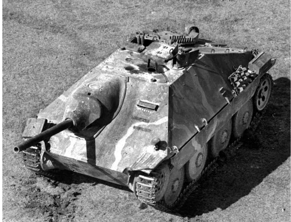
ABOVE: The compact Jagdpanzer, just under 7 feet tall, was most effective firing its armor-piercing and high-explosive shells at the flanks of enemy armored formations from hidden positions. BELOW: Jagdpanzer 38 assembly line in Böhmischem-Mährische Maschinenfabrik AG plant, June 19 1944. Škoda along with B.M.M. assembled about 2,827 Jagdpanzer 38(t).
