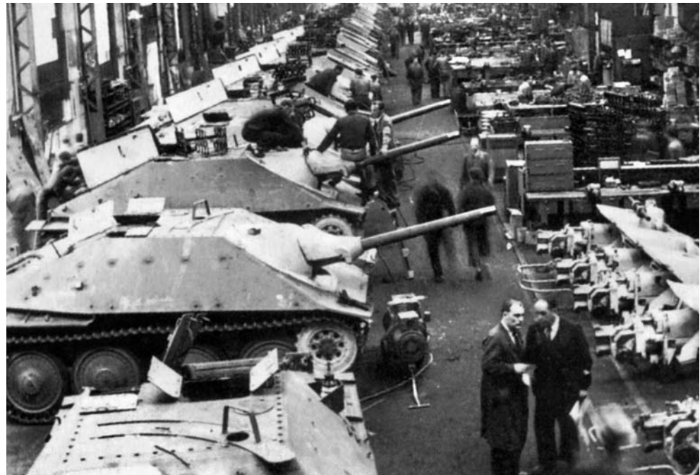
ABOVE: The compact Jagdpanzer, just under 7 feet tall, was most effective firing its armor-piercing and high-explosive shells at the flanks of enemy armored formations from hidden positions. BELOW: Jagdpanzer 38 assembly line in Böhmischem-Mährische Maschinenfabrik AG plant, June 19 1944. Škoda along with B.M.M. assembled about 2,827 Jagdpanzer 38(t).
