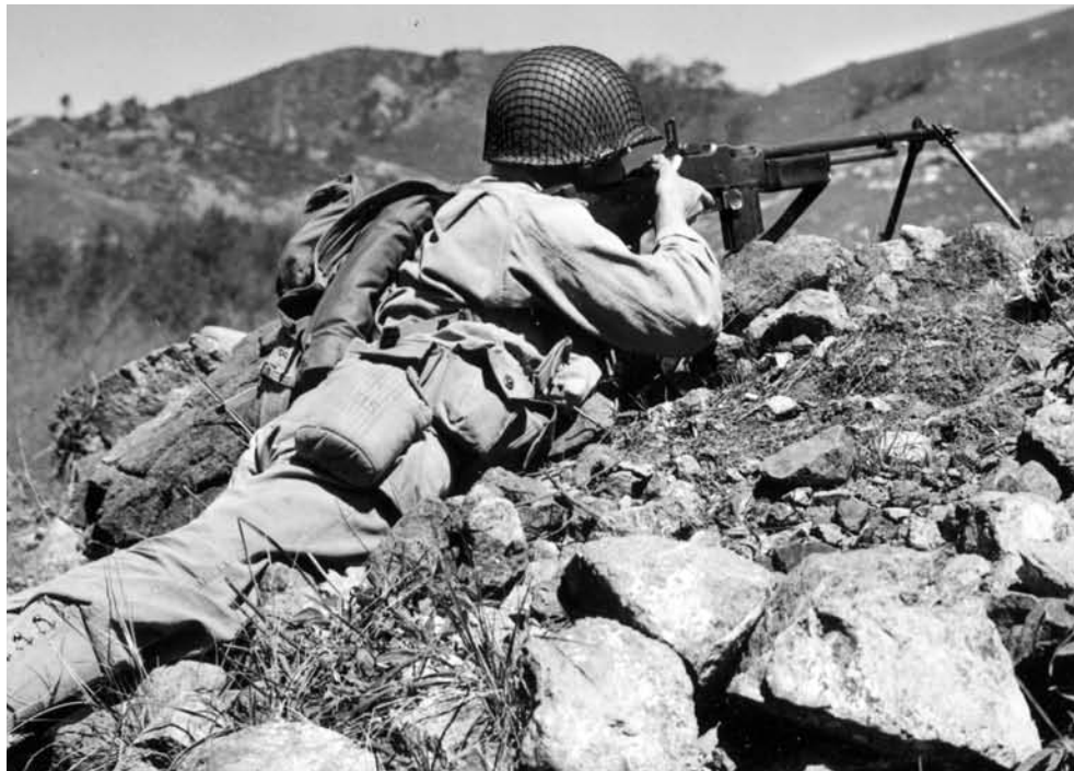
To stabilize the BAR when used in the prone position, military contractors produced a bipod and a hinged bullet plate in 1937 for the M1918A1 version. The venerable BAR, which saw use from World War I to the early days of the Vietnam War, served U.S. ground forces well.
