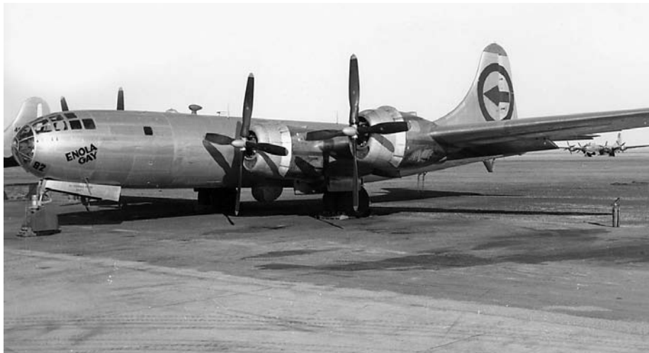
ABOVE: The four engine B-29 Superfortress Enola Gay sits on an airfield tarmac. The bomber’s tricycle landing gear is plainly visible in this photo. The B-29 featured numerous innovations, including a pressurized cabin. BELOW: Colonel Paul Tibbets tackled numerous assignments during a long Air Force career.
