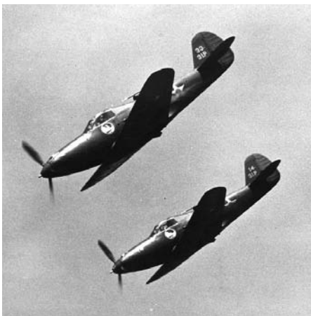
ABOVE: Though the P-39 lacked high-altitude capabilities, its short wingspan and tight turning radius made it particularly effective when used in a ground support role. BELOW: Sporting Red Air Force markings, this P-39 Airacobra is typical of the approximately 5,000 such fighters supplied to the Soviets during the Lend-Lease program by way of Alaska.
