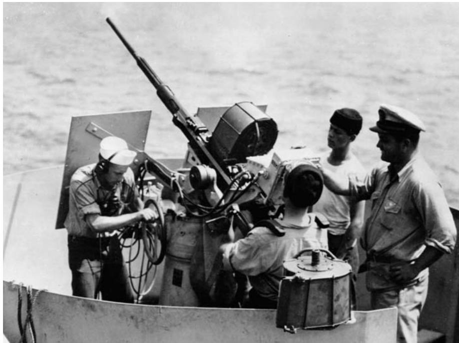
A 20mm Oerlikon cannon is shown in action aboard the destroyer escort USS Jacob Jones .
