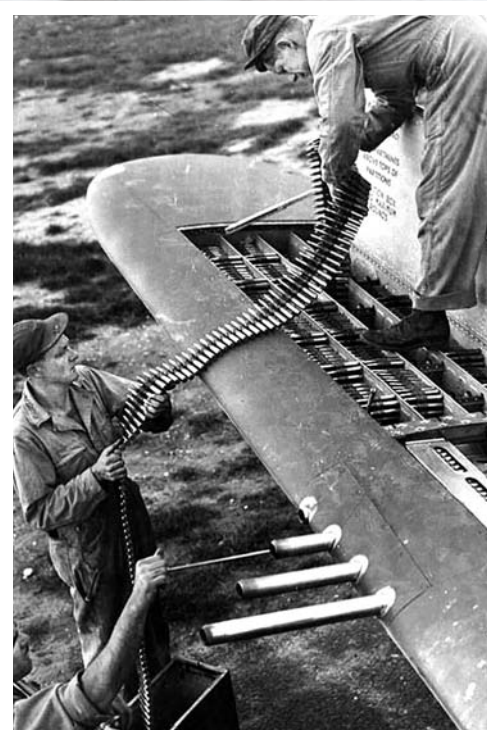
With its huge Pratt & Whitney R-2800 Double Wasp radial engine, a bulky P-47D Thunderbolt like “Torrid Tessie,” seen here flying over Italy in 1945, could carry eight Browning .50 caliber machine guns and 3,200 rounds—more than any other plan in the war. INSET: Armorers load .50 caliber ammunition belts into the four ammo trays of a P-47 Thunderbolt.
