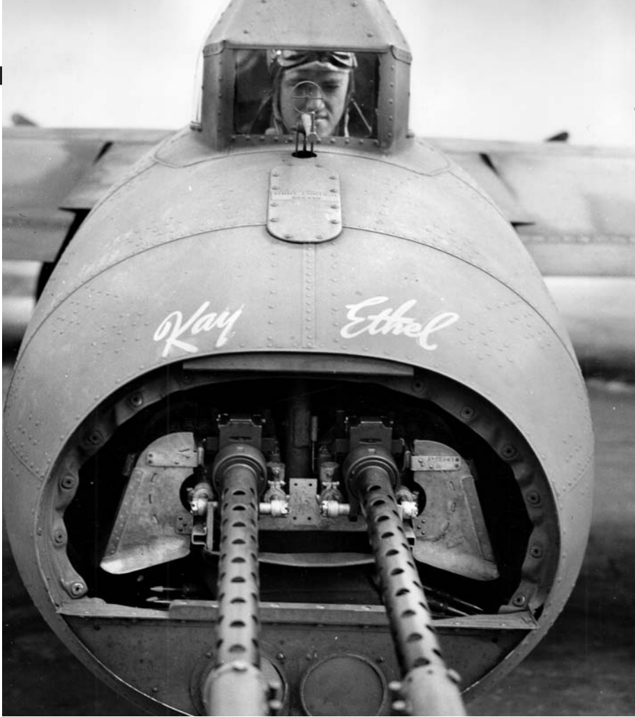
ABOVE: The tail gunner on the B-17 "Hell's Angels" poses for a photo with his twin .50-caliber machine guns between missions. Tucker said that he once had to shake his guns at a USAAF rookie pilot who flew too close to his "office." OPPOSITE: At Amendola Field a stretcher crew (under fuselage) works to remove a casualty from a 97th Bomb Group B-17 "Marishka" after it returned from a combat mission. Tucker noted that after each mission a medic offered crews a shot of whiskey to help them through post-raid debriefings.
