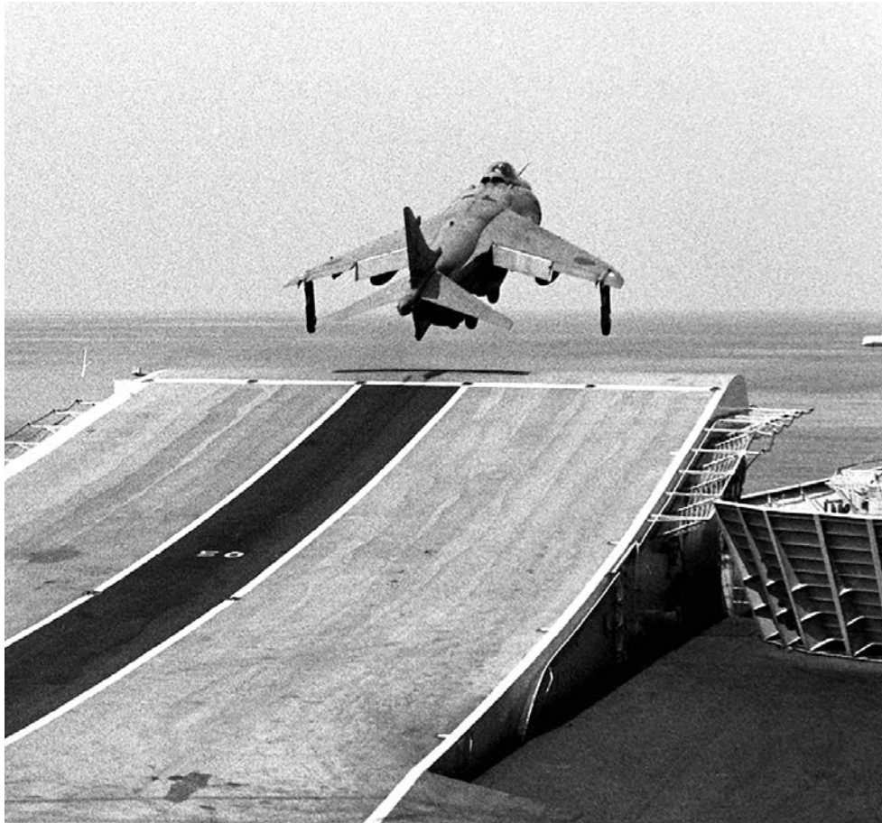
ABOVE: An FRS. Mark 1 Sea Harrier aircraft takes off from the flight deck of the British light aircraft carrier HMS Invincible during the NATO Southern Region exercise “Dragon Hammer” in 1990. An upward-curved ramp angled at 6.5 degrees allowed Sea Harriers to take off with a higher disposal payload. OPPOSITE: Sea Harrier FRS.1s XZ451 (foreground) and ZA176 flying in “Operation Corporate,” the former using its AIM-9L Sidewinders, which it is seen carrying here, to shoot down several Argentine aircraft, including a Canberra B-108 bomber on May 1, 1982, and a C-130 Hercules transport on June 1.
