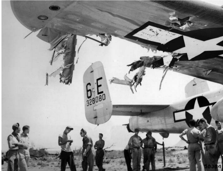
ABOVE: This North American B-25 Mitchell bomber took a direct hit from German flak over southern France but managed to land safely at its base during the harrowing 1944 mission. The damage to the right wing is extensive, as evidenced in the photo. OPPOSITE: A squadron of B-25 bombers speeds its way toward a rail yard, the target of this mission during the Italian campaign. The B-25s regularly bombed rail yards in northern Italy to prevent the movement of German reinforcements and equipment toward the front lines to the south.
