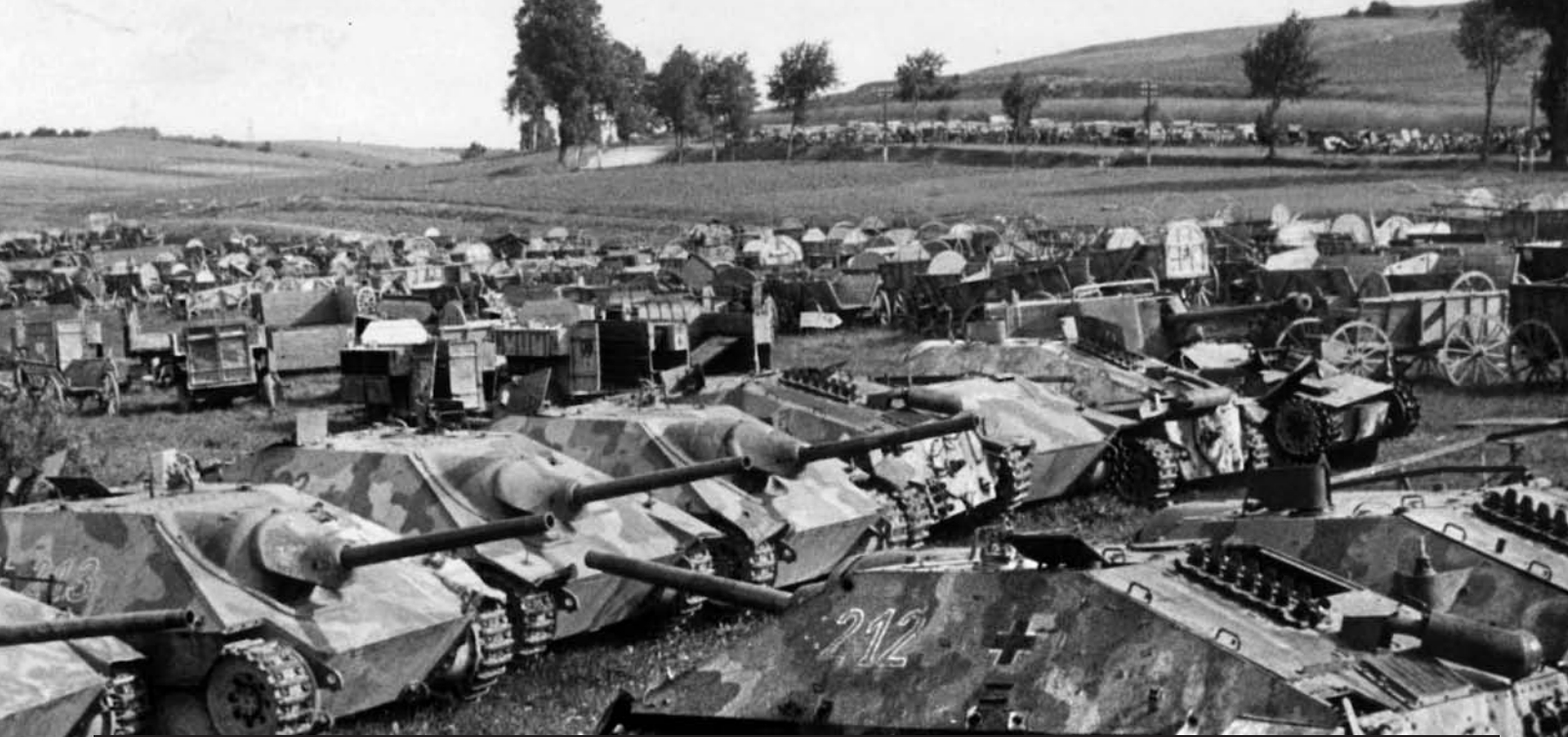
These captured armored vehicles were surrendered to the Soviet Red Army in 1945. Among them are several examples of the Panzerjäger 38(t) assault gun, popularly known as the Hetzer and built on the Czech 38(t) chassis. Also built on the Czech 38(t) chassis, a Marder III is visible at right. Horse-drawn wagons are shown toward the rear.
