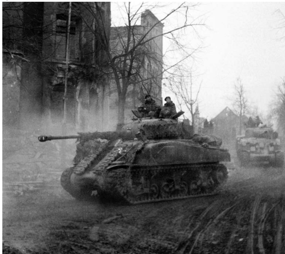
ABOVE: Sherman Firefly tanks moving through Cleve in the Rhineland on February 16, 1945, on the way to take the town of Goch. A British innovation, the Firefly was an M4 Sherman fitted with a high-velocity 17-pound (76.2mm) gun more suited for combat against other tanks. OPPOSITE: British soldiers cross the Niers River on March 2, 1945, heading for the nearby town of Weeze, Germany. The Germans disabled dams to allow normally small rivers to overflow their banks. Some floodwaters took as long as two weeks to recede.
