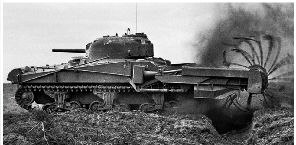
A problem solving engineer, Major General Percy Hobart developed the "Crab" from a Sherman tank with a chain flail attached to detonate mines. His "Crocodile," fashioned from a Churchill tank, was fitted with a flamethrower and towed a 400-gallon armored fuel tank for it.
