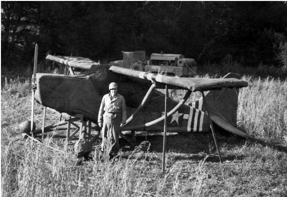
An inflated rubber L-5 reconnaissance plane used by the Ghost Army at one of the last operations on the western border of Germany.
