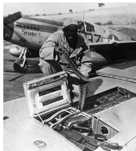
ABOVE: On January 12, 1944, a row of Mustangs fills an assembly line at the Consolidated Vultee aircraft manufacturing plant in Tucson, Arizona. The Mustang served in both the European and Pacific Theaters during World War II. RIGHT: A Fifteenth Air Force armorer loads a belt of ammunition for one of a Mustang's six .50-caliber machine guns. Flying from its base in Italy, this fighter plane was being readied for a mission over Germany. Often, when escort duties were completed, the Mustangs were allowed to seek targets of opportunity.
