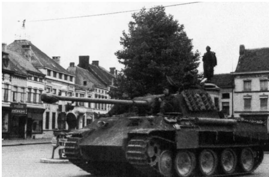
Pausing momentarily in the square of a deserted French town, a Panther medium tank and its 75mm high velocity cannon present a menacing profile. The Panther was designed by German engineers in response to the hugely successful Soviet T-34. (National Archives)
