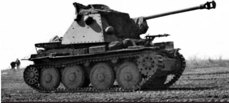
This self-propelled gun, a variant of the Marder, includes the Czech-designed 38(t) chassis. It mounts a powerful 75mm cannon and a 7.62mm machine gun for defense against infantry attack.
