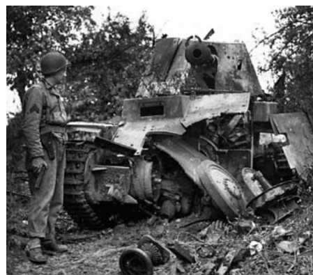
An American soldier inspects the hulk of a Model M Marder that has been disabled by a direct hit against its chassis from an Allied artillery shell.
