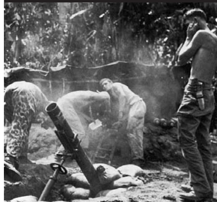
A 4.2-inch chemical mortar is fired by its U.S. Army crew on the island of New Britain in the Pacific near the great Japanese base at Rabaul. The 4.2-inch chemical mortar provided essential firepower and smoke-generating capabilities for frontline troops.
