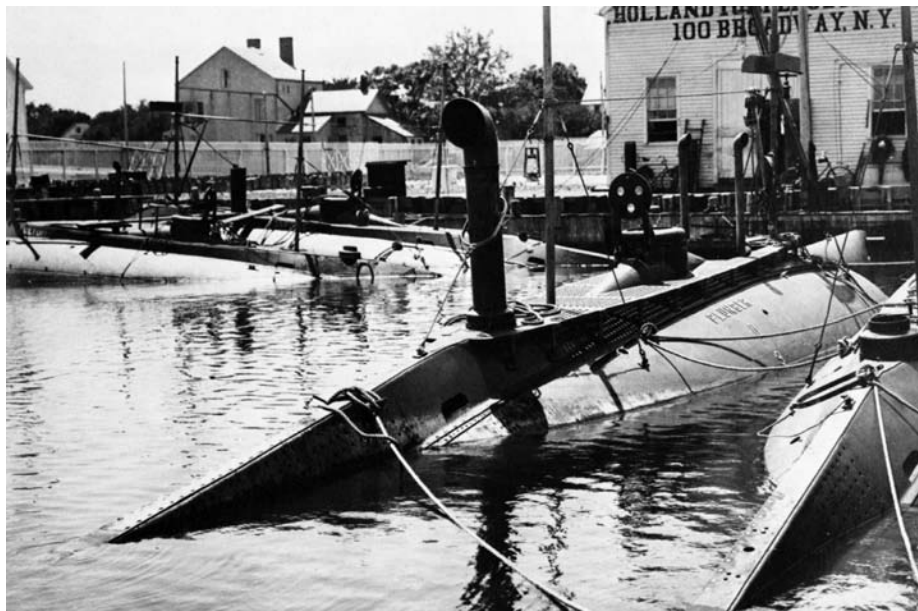
ABOVE: Five submarines built by the Holland Torpedo Boat Company ride at anchor at a New York dock in 1902. Plunger , center, was an improved version of Holland . TOP: The submarine Holland was constructed by the Crescent Shipyard in Elizabeth, New Jersey, and was commissioned by the Navy in April 1900.
