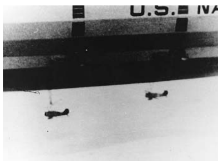
ABOVE: Two F9C-2 Sparrowhawks are attached to the Macon ’s underbelly during this 1934 flight. TOP: In flight, a biplane tests the hook-on device attached to the bottom of the USS Akron .
