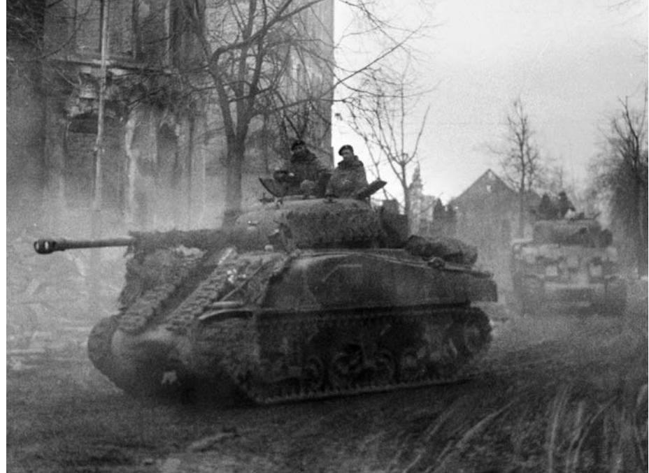
ABOVE: Sherman Firefly tanks advance through the ruins of Kleve during an attack on the nearby village of Goch on February 16, 1945. The Firefly was a British innovation that replaced the original 75mm cannon of the M4 Sherman with a high-velocity 17-pounder (76.2mm) gun which was more capable in tank versus tank combat. OPPOSITE: Wary British troops of the 2nd Gordon Highlanders scan windows for German snipers in the town of Kleve.
