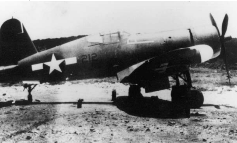
The long fuselage, distinctive gull wings, and radar installation on the right wing of the Vought F4U-2 Corsair night fighter are visible in this photograph.
