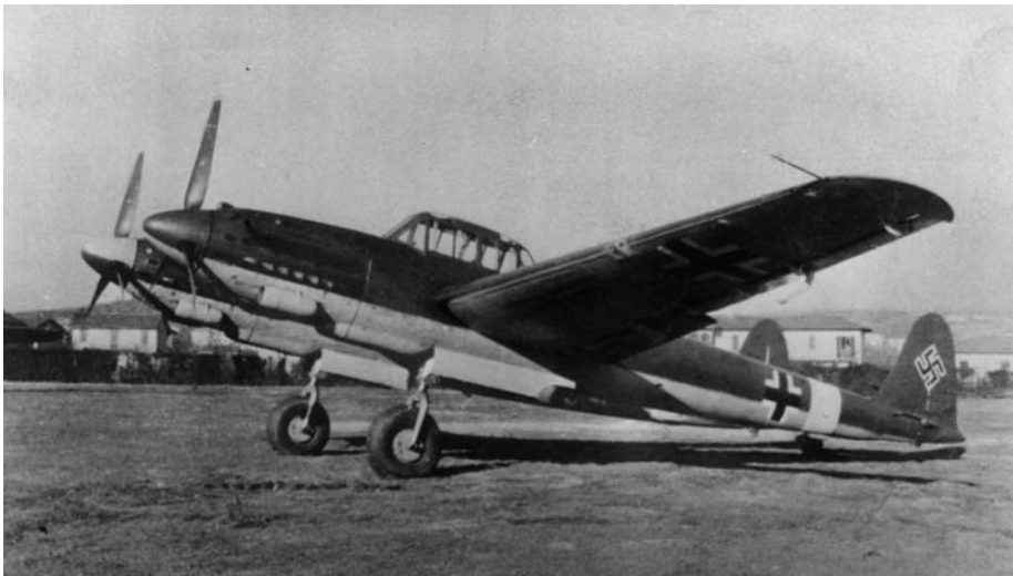
The SM.92 moved the cockpit to the portside engine boom and added five 12.7mm machine guns. It was faster than the SM.91 and had more range.
