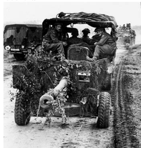
ABOVE: The British six-pounder could reliably pierce the armor of any tank the Germans could field in the deserts of North Africa. RIGHT: British troops move forward on the Argentan road in August 1944, with antitank weapons in tow. Heavier antitank weapons were welcome in combat against the German Mark V Panther and Mark VI Tiger tanks.
