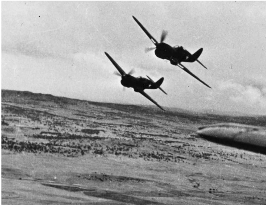
A pair of Curtiss P-40 Warhawk fighter planes is shown during a training exercise in Australia. The heavy P-40 could outdive the nimble Japanese Zero, and experienced pilots learned to take a single pass at the enemy fighters from a position above the target.
