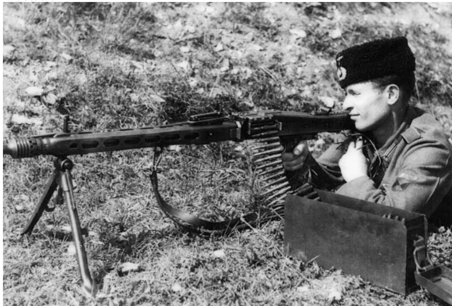
A Cossack soldier trains with the German MG-42 machine gun. The MG-42 was known for its high rate of fire and distinctive sound on the battlefield. Bullets are being fed directly from the adjacent ammunition box.
