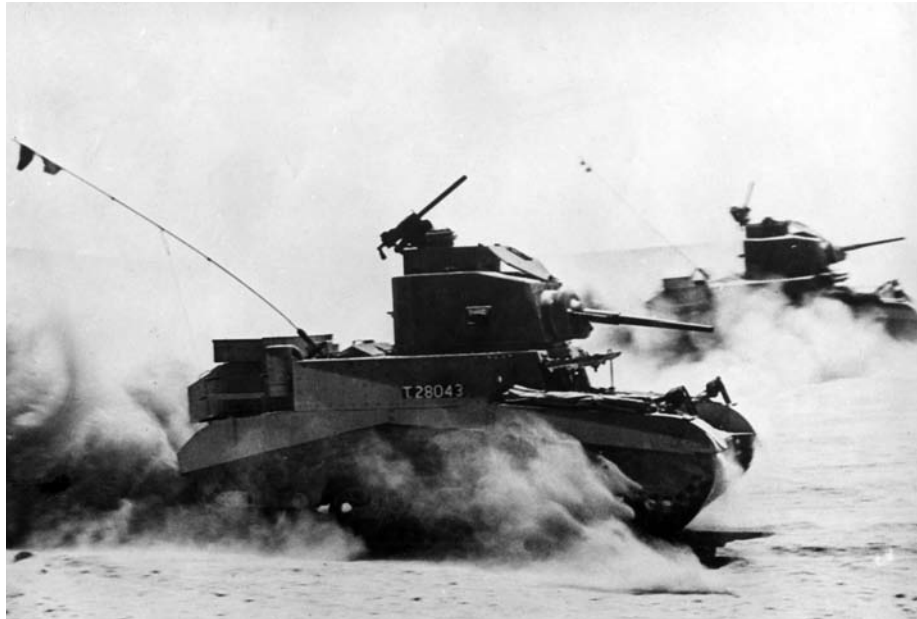
Newly delivered Stuart tanks undergo testing in the North African desert. Later, the U.S. supplied the heavier M3 Lee tank, with a sponson-mounted 75mm gun in the hull and a turret-mounted 37mm cannon.
