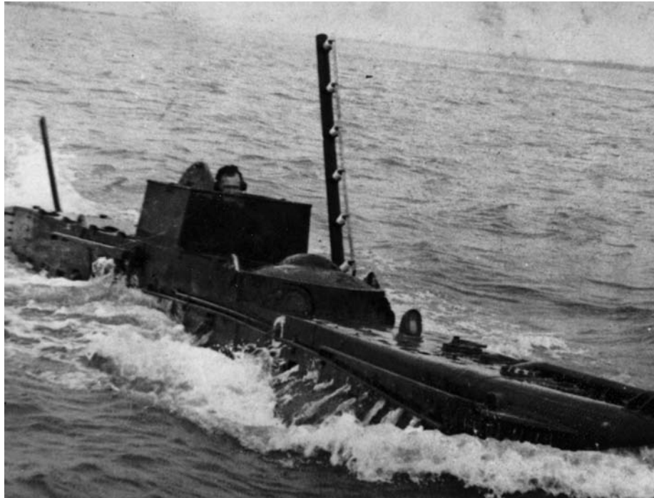
A prototype X-craft churns along during trials. Although it experienced some navigational and mechanical challenges, the midget submarine proved well suited for the attack on Tirpitz .
