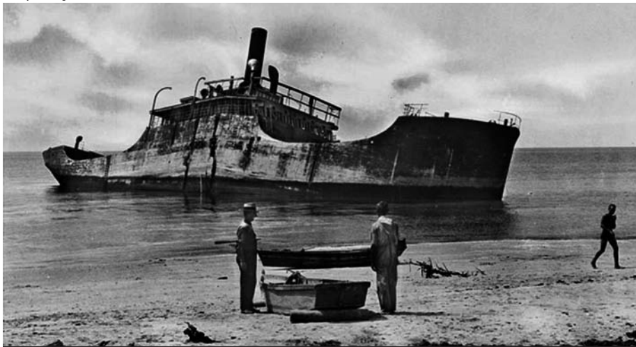
The forlorn hulk of the SS Atlantis lies off Cape May, New Jersey. Launched on December 5, 1918, Atlantis was the second concrete ship built in the United States. The vessel was used to transport American soldiers home from World War I and ran aground in 1926.
