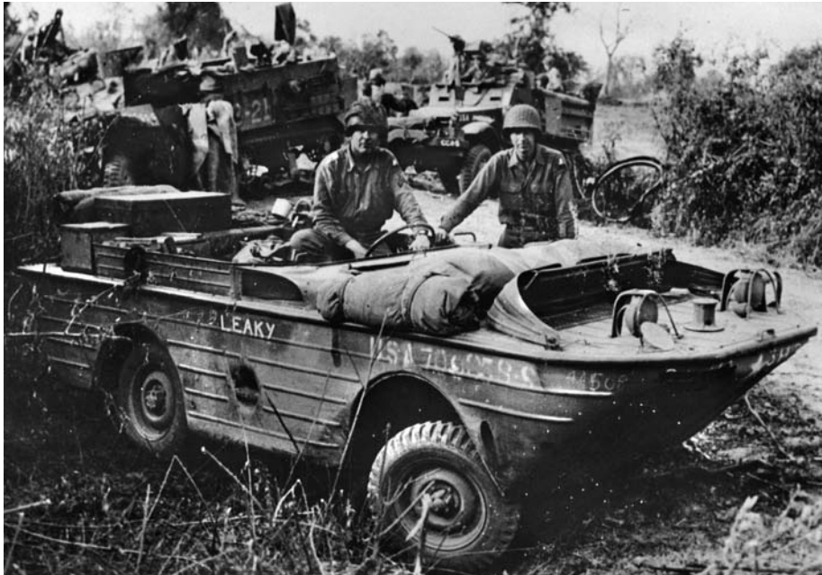
The seep, an amphibious variant of the jeep, is shown in the field in 1944. These troops have taken the seep in swampy conditions that require a vehicle capable of gaining traction in difficult terrain.
