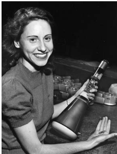
A female researcher holds a conventional 5-inch cathode ray oscilloscope in her left hand and a sub-miniature radio tube in her right.
