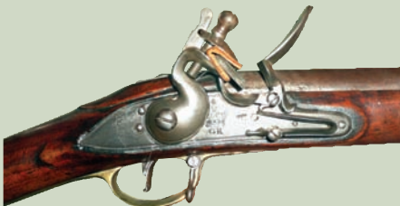
Close-up view of flintlock, with the flint wrapped in a strip of leather in the jaws of the cock.
