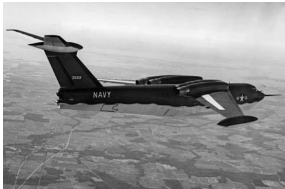
Early tests of the Martin XP6M-1 SeaMaster showed that its engines scorched the fuselage. Four crewmen were killed on a routine test flight in 1955.
