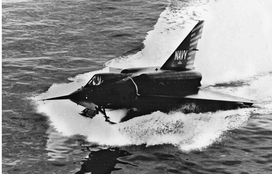
ABOVE: The Convair XF2Y-1 Sea Dart takes off in the water on retractable skis. During its first public demonstration the plane disintegrated in mid-air, killing the pilot. BELOW: The Convair R3Y-1 Tradewind, nicknamed the Flying LST, was intended to operate as a landing craft, but it performed more efficiently as an aerial tanker.
