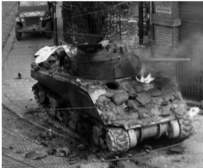
LEFT: An abandoned American Sherman tank, destroyed by a direct hit from a German Faustpatrone, hollow-charge projectile, sits on a street in Leipzig, Germany. BELOW: Some M4 tanks were equipped with 4.5-inch rocket launchers and dubbed Calliopes. Although the rockets were inaccurate, they could saturate a significant area with high-explosive ordnance.
