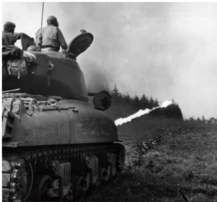
A Sherman tank modified to carry a flamethrower demonstrates its usefulness against enemy fixed fortifications in September 1944.
