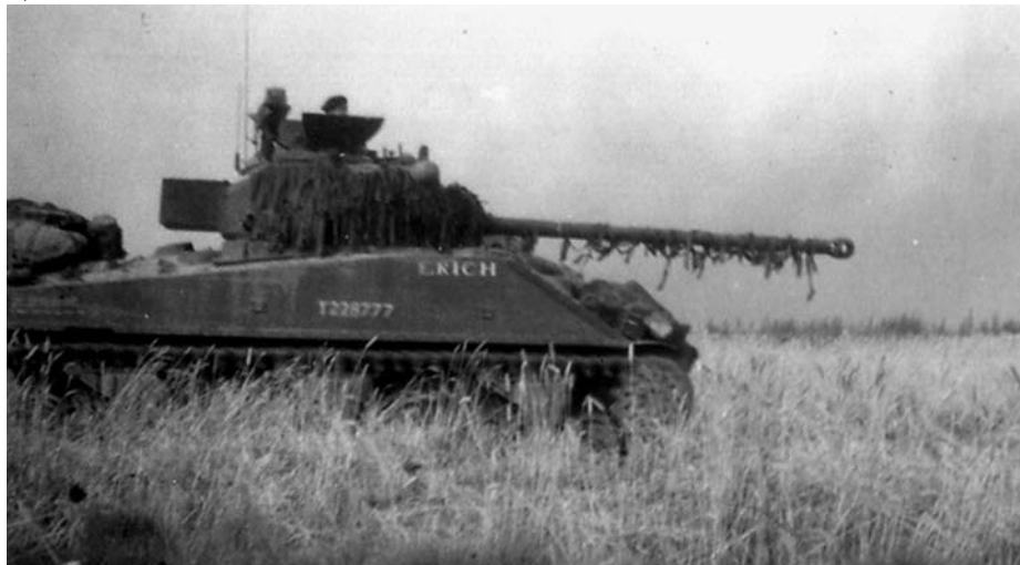
Photographed in July 1944, this camouflaged Canadian Sherman is known as the Firefly. These Shermans were upgunned with the British 17-pounder to help even the odds against German armor.
