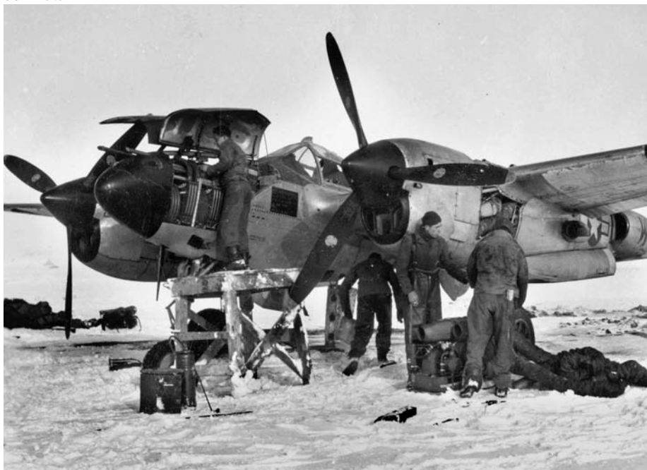
ABOVE: Ground crewmen use an external heater to warm up one of the twin engines aboard a Lockheed P-38 Lightning fighter of the Ninth Tactical Air Force. An armorer loads the guns in the nose of the fighter plane. BELOW: Rugged Republic P-47 Thunderbolt fighter bombers of the 365th Group take off on a tactical support mission during the Battle of the Bulge. OPPOSITE: A rain of ordnance from Allied Eighth Air Force heavy bombers demolishes the rail yard at Euskirchen, Germany, on December 23, 1944.
