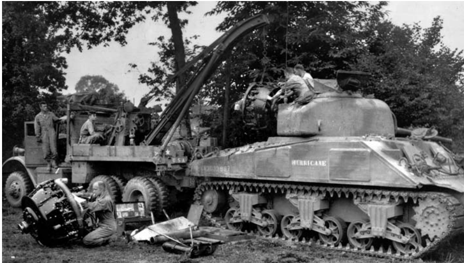
Still tethered to its recovery vehicle, an M4 Sherman tank nicknamed Hurricane has its engine overhauled in the field. One of the virtues of the lightly armored Sherman was its reliability and the fact that such maintenance could be accomplished in less than ideal conditions near the front.
