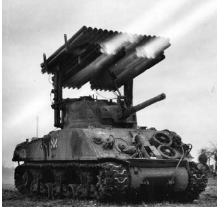
LEFT: An abandoned American Sherman tank, destroyed by a direct hit from a German Faustpatrone, hollow-charge projectile, sits on a street in Leipzig, Germany. BELOW: Some M4 tanks were equipped with 4.5-inch rocket launchers and dubbed Calliopes. Although the rockets were inaccurate, they could saturate a significant area with high-explosive ordnance.
