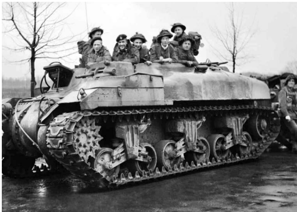
ABOVE: Manufactured from the modified chassis of the M4 Sherman medium tank, this Kangaroo personnel carrier transports soldiers of the 53rd Welsh Division during the Battle of the Reichwald in February and March, 1945. TOP: On February 13, Private A. Rees of the 2nd Gordon Highlanders, 15th (Scottish) Division, cleans his Lee-Enfield Mark IV, No. 1 rifle in the ruins of building in Kleve, Germany, near the Dutch border.
