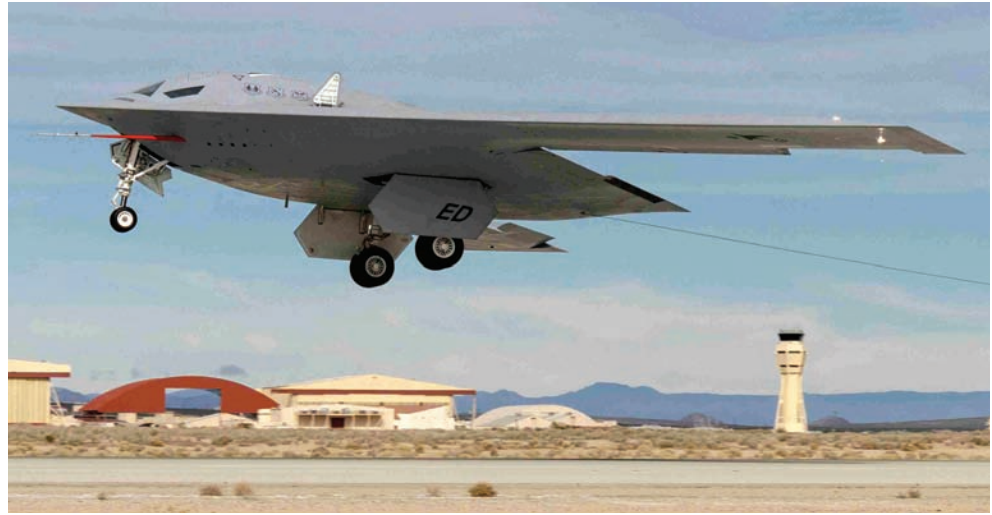
The next generation stealth bomber—the B-21 Raider—on a test flight at California’s Edwards Air Force Base. The B-21 will have a shorter wingspan and smaller payload than the B-2, but its radar-absorbent material (RAM) coating will make it even more difficult to detect.
