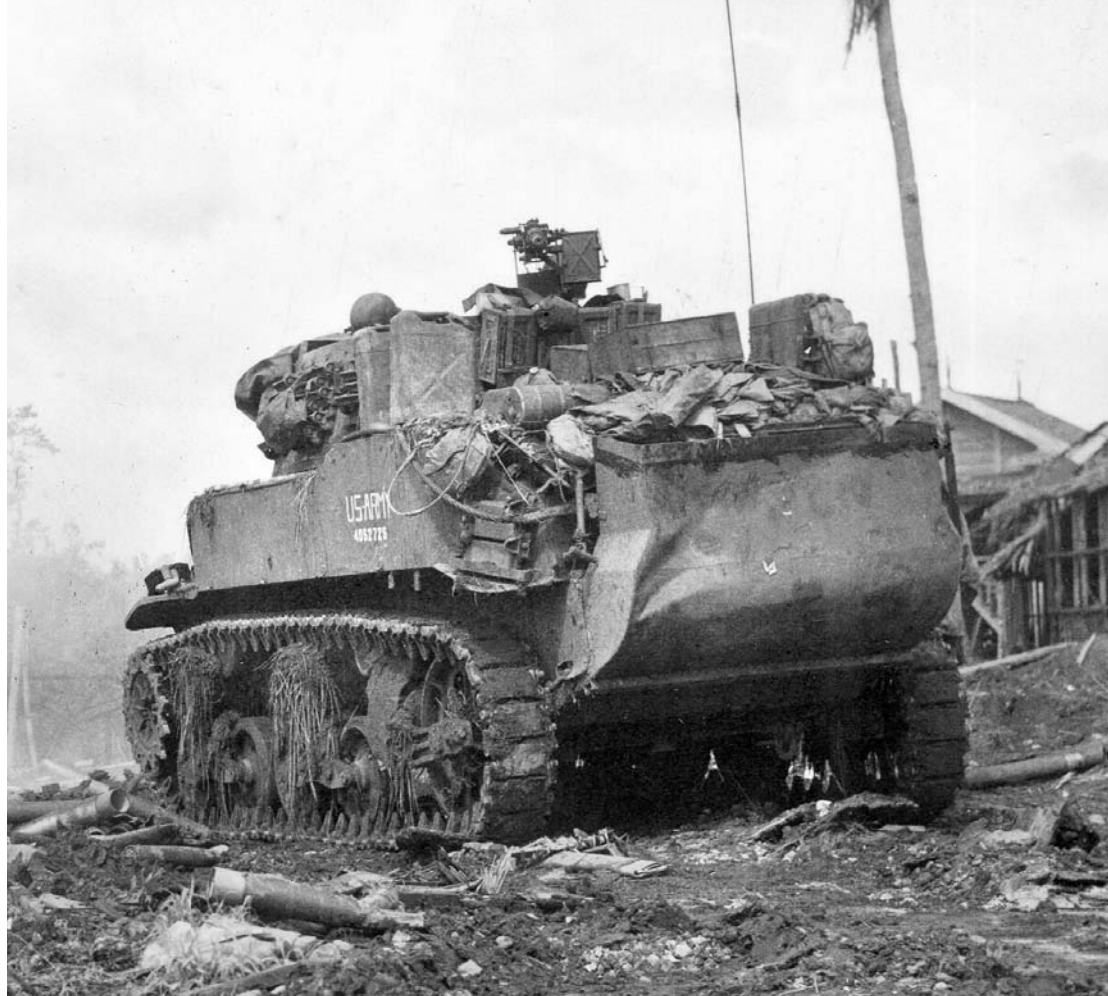
A U.S. Army M8 self-propelled gun fires on a Japanese pillbox in support of the 77th Infantry Division fighting in the Ormoc Valley on west Leyte Island in the Philippines. Equipped with snorkels during landings, the Howitzer Motor Carriage M8 could land in shallow water and proved effective in the Pacific War.
