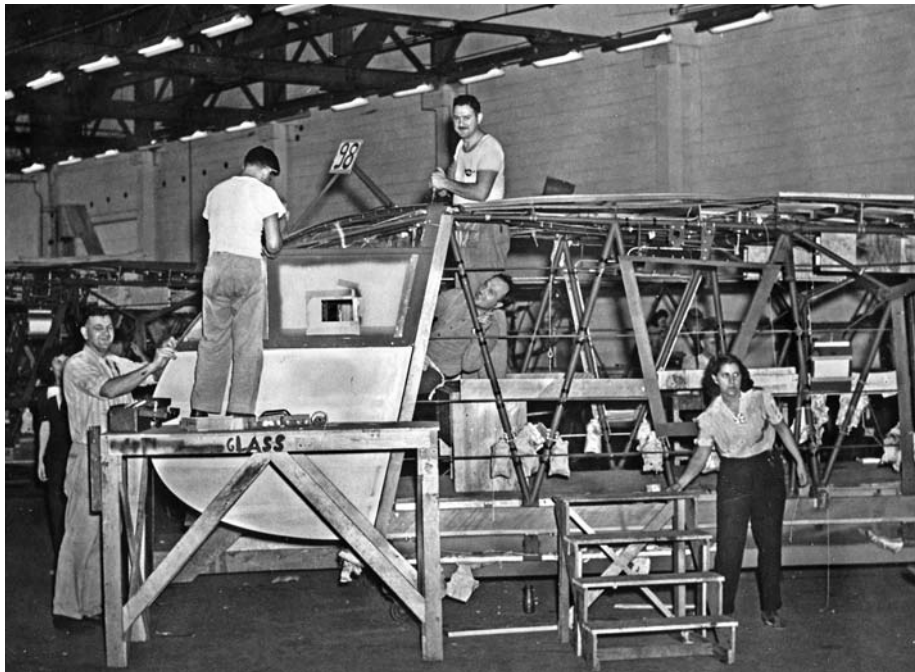
Pratt, Read employees perform primary assembly work on a Waco CG-4A glider. With over 70,000 parts, the CG-4A proved almost impossible for manufacturers with little or no aircraft-making experience to build.
