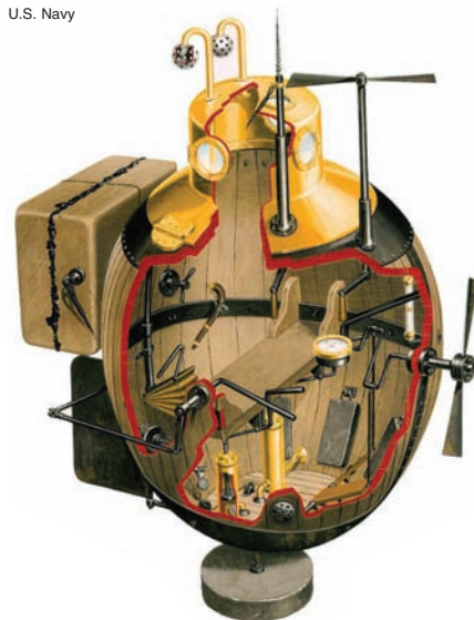
ABOVE: Cutaway of Revolutionary War-era Turtle .
