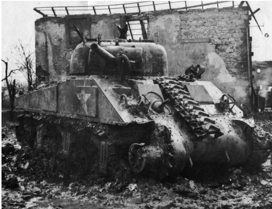
This Sherman tank commanded by Sergeant Giles W. Hayward was hit twice by German shells during the fight at Singling. The second shell struck the Sherman in its right sprocket, blowing off the tread and crippling the tank.
