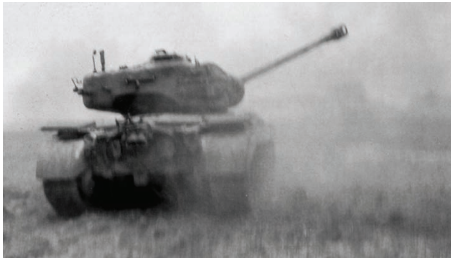
ABOVE: An M26 in action near the Rhine River in March 1945. The M26 Pershing heavy tank entered development with the U.S. Army in mid-1942, just as full production of the medium M4 Sherman tank was getting under way. BELOW: One of the M26 tanks from the 14th Tank Battalion that supported the capture of the Ludendorff Bridge over the Rhine on March 7, 1945.
