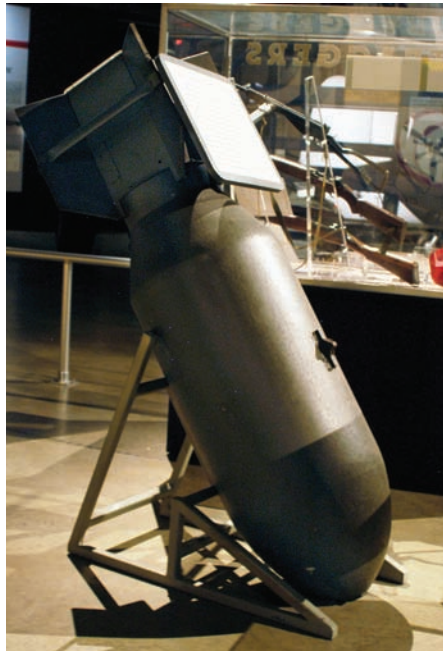
The initial variant, the Vertical Bomb-1, used a 1,000-pound bomb with a modified tail unit. This one is on display at the National Museum of the U.S. Air Force in Dayton, Ohio.
