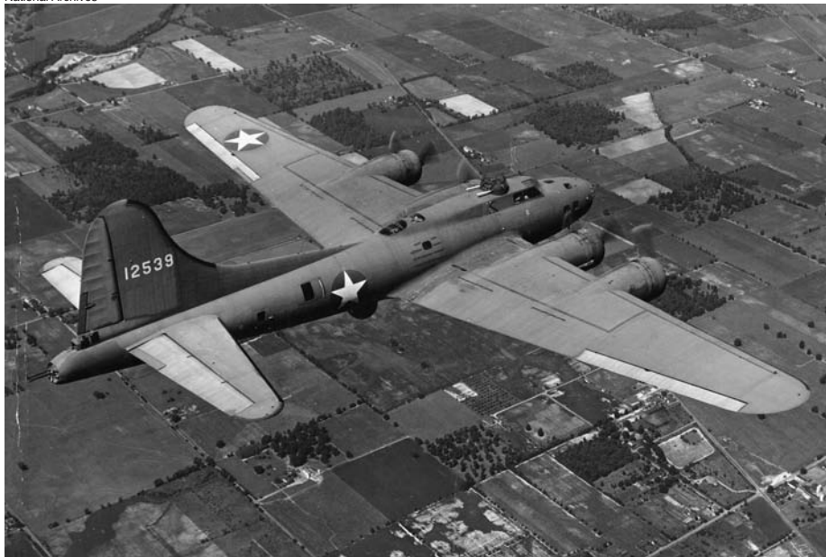
Photographed in 1943, this image of a new Boeing B-17 Flying Fortress bomber presents an excellent view of the four-engine aircraft that was instrumental in prosecuting the air war against Nazi Germany. The tail gunner's position is visible at lower left.
