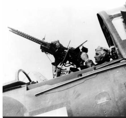
ABOVE: Jim Samar, a radio operator/gunner with dive bombing squadron VB-80, sits in the back seat of a Curtiss SB2C Helldiver and demonstrates taking aim with the twin mounted .30-caliber (7.62mm) machine guns installed to ward off enemy fighter planes. BELOW: This U.S. Navy Curtiss SB2C Helldiver is releasing its bomb during a training run. Note that both the pilot's and the gunner's canopies are open.
