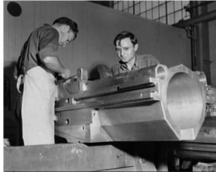
Workmen on the floor at the Watervliet Arsenal finish the breech housing for a medium caliber gun at the Watervliet Arsenal. Hundreds of workers were employed at the arsenal during the war years.
