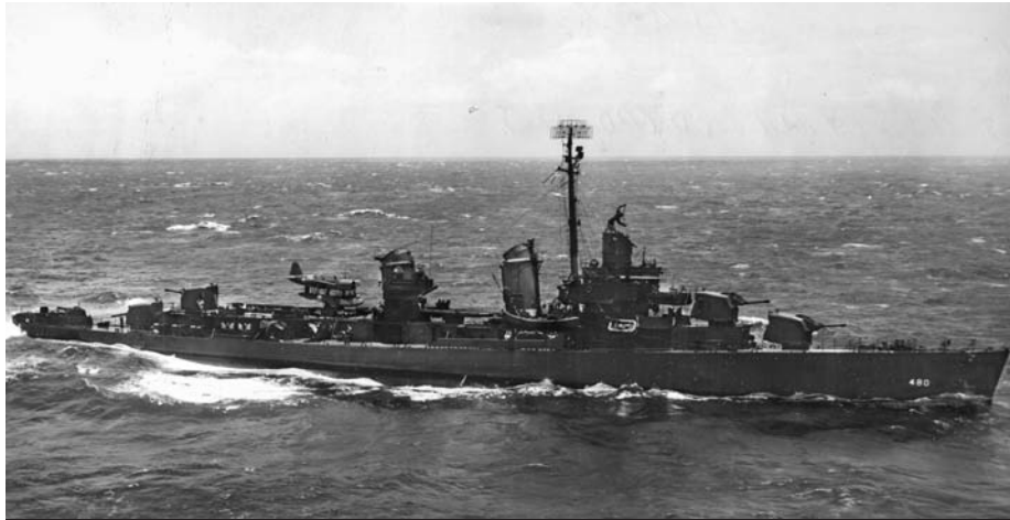
The Fletcher-class destroyer USS Halford was one of the warships equipped with a catapult. The Halford is shown at sea with its Vought Kingfisher aircraft and catapult (circled) in place.
