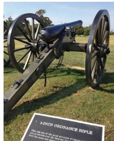
A 3-inch Rifle on display at Antietam National Battlefield. The guns fired 9-pound Hotchkiss or Schenkl projectiles and also could accommodate 10-pound Parrott projectiles.
