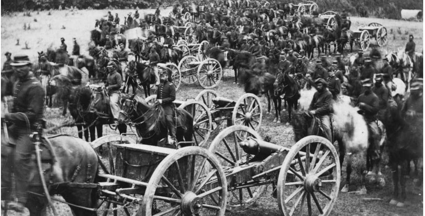
A battery of 3-inch Rifles during the Peninsula Campaign in 1862. Although no match for the 12-pounder, bronze smoothbores in close-range action, the 3-inch rifle had a significantly lighter barrel that made the cannon easier to move.
