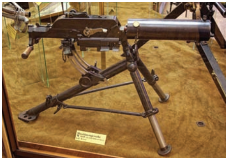
The simple design of the water-cooled Austrian Schwarzlose M.07/12 World War I-era medium machine-gun was well suited for mass production.
