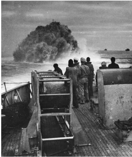
The crew of USCGC Spencer watches the results of a direct hit with a depth charge on U-175 in April 1943. Allied naval personnel found that resetting depth charges to explode at 25 feet rather than 100 feet resulted in more kills.
