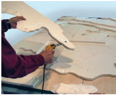
The terrain board, which is based on a modern topographical map, is built up with layers of Styrofoam insulation board. Once it has been sculpted with a hot knife into an accurate representation of the terrain, the Styrofoam is covered with cloth and painted to replicate the landscape at the time of the battle.
