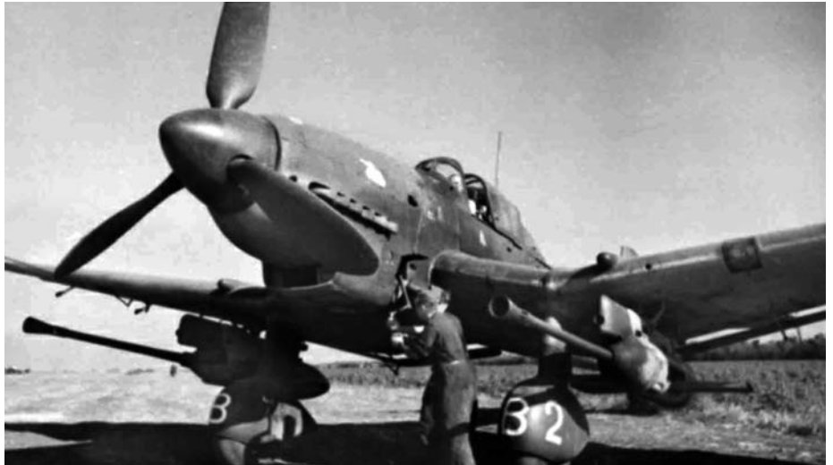
Rudel’s Stuka “Gustav” mounting twin 3.7cm cannon under the wings is prepared for a sortie in Russia. The tank-killer version was even slower and less maneuverable than the dive-bomber version, but Rudel nevertheless achieved impressive results with it.
